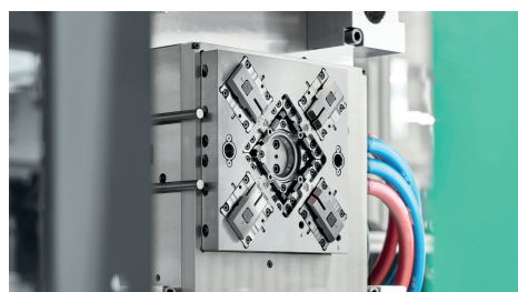
Fig. 5. Luer connectors with molded-on septum on the lid. This is closed while still in the mold by means of a sophisticated mechanism. © Arburg
