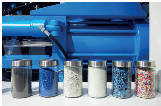
Fig. 8. Three recyclates of different viscosities, plus three kinds of additives, are processed in one heating step by the DCIM process.
